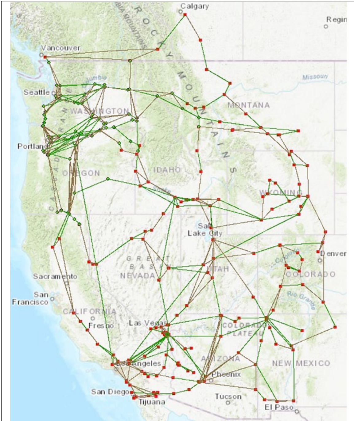
Figure 1. WI system map. Green circles represent BPA buses and red squares represent buses outside the BPA area. Service Layer Credits: Sources: Esri, HERE, DeLorme, Intermap, increment P Corp., GEBCO, USGS, FAO, NPS, NRCAN, GeoBase, IGN, Kadaster NL, Ordnance Survey, Esri Japan, METI, Esri China (Hong Kong), swisstopo, MapmyIndia, © OpenStreetMap contributors, and the GIS User Community.
